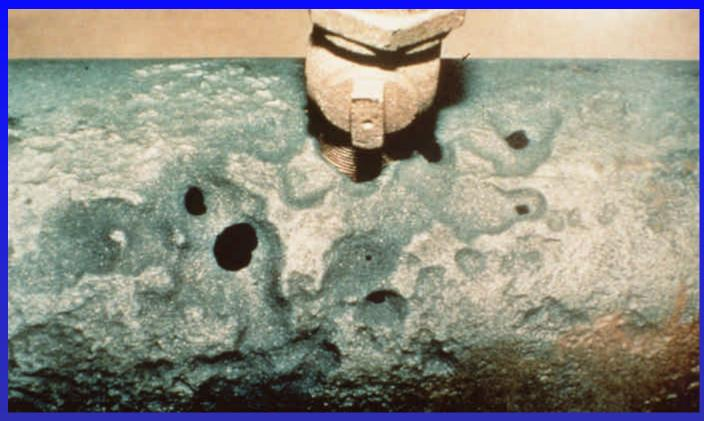
Corrosion of iron when coupled to copper service line.
