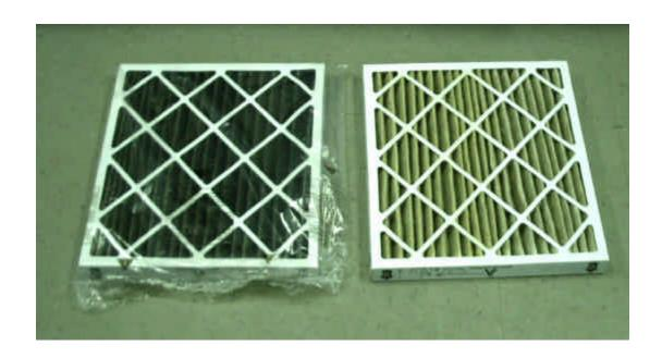
Picture showing the difference between new and used filter utilized to purify incoming air at SLOAN KETTERING Cancer Research Center. Filter has turned black due to Diesel soot emissions from city buses which stop near air intake.
